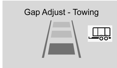
Near Gap Setting with Trailer
