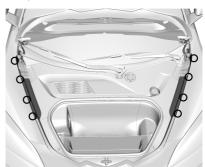
Release the four clips for the left and right outer covers.
