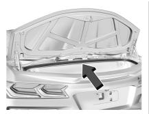
Use the pull cup to lower the hatch if needed, then drop into the latch or push on the outside of the panel until the power latch feature activates. The hatch/trunk will close the rest of the way and latch automaticallu.
