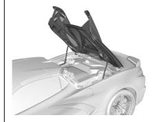
Hold until the tonneau cover is completely opened. The turn signals will flash once
