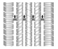
Treadwear indicators are one way to tell when it is time for new tires. Treadwear indicators appear when the tires have only 1.6 mm (1/16 in) or less of tread remaining. See *Tire Inspection* ⇒ 278 and *Tire Rotation* ⇒ 279.
