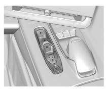
This vehicle is equipped with a dual clutch transmission that contains an integrated rear differential. The dual clutch transmission provides an extremely connected feel due to the direct connection between the engine and gear box. This arrangement provides very fast shift times for maximum performance. Automatic driving mode is selected by pulling D on the transmission range selection panel and
