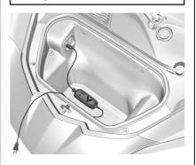
Some vehicles have a battery maintainer package. Follow the instructions provided with the battery maintainer package to keep the battery charged when the vehicle is not in use. Plug the battery maintainer into the underhood accessory power outlet only.
