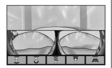
If equipped, a view of the area in front of the vehicle displays in the infotainment display. The display shows a front, top down view at the top and left and right front camera images on the bottom. The front view shows after shifting from R (Reverse) to a forward gear, or by pressing the camera button on the center console, and when the vehicle is moving forward slower than 12 km/h (8 mph).
