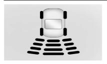
The instrument cluster may have a Park Assist display with bars that show "distance to object" and object location information for RPA. As the object gets closer, more bars light up and the bars change color from yellow to amber to red.
