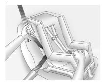
To tighten the belt, push down on the child restraint, pull the shoulder portion of the belt to tighten the lap portion of the belt, and feed the shoulder belt back into the retractor.
