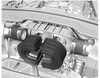
Remove the air cleaner filter(s) (top image LT2 engine) (bottom image LT6 engine).
