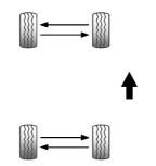
Use this rotation pattern if the vehicle has different size tires on the front and rear.
