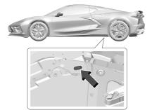
Use only a service jack with a lifting pad diameter of 64 mm (2.5 in) or smaller, and thick enough to make sure the jack does not contact the vehicle body.
