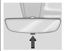
Pull the tab to turn on the display. Push the tab to turn it off. When the display is off, the automatic dimming function is active.
