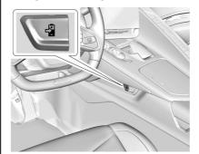
Press the Charge+ button on the drive side of the center console. When the Charge+ feature is active, the hybrid battery charging light displays on the DIC. See *Hybrid Battery Charging Light* \$4. Also, a small pop-up window will also appear showing the exact SOC and electric power input/output. The
