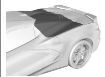
5. Hold am until the tonneau cover is completely closed. A chime will sound, a DIC message will display, and the turn signals will flash once.
