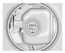
When the engine is cold, the coolant level should be at the COLD FILL indicator in the coolant surge tank.
