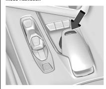
To activate My mode, Weather, Tour, Sport and Track mode, turn the DMC knob on the center console to make a mode selection. When a mode is selected, an indicator will
