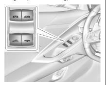
Press to lower the midglass. To provide wind block, the midglass will not lower completely. The midglass will also lower automatically when lowering the convertible top.
