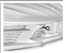
Install the tow eye into the socket and turn it until it is fully tightened.
